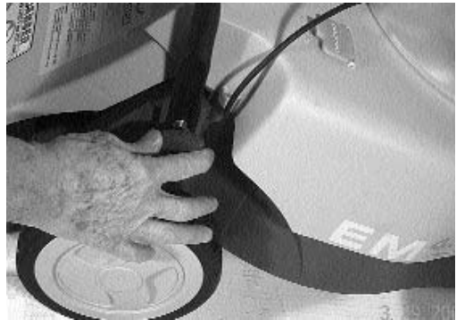
Figure 6. Tighten the green quick-connect knobs
